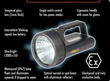
MICA IL-80 ATEX LED is a rugged, high-performance flashlight for explosion-hazardous areas. With its ergonomic dual-mode switch the user can choose between a 21h operating time and two light output modes. The construction of the MICA IL-80 ATEX LED is designed for easy servicing and for an extremely long working lifespan. End-user can easily perform most services.
